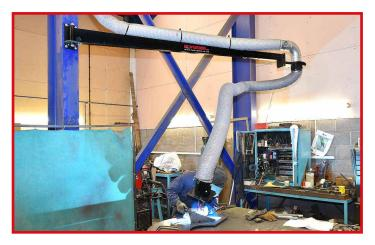
Both the Flexi weld arms and Flexi crane arms are easy to use and ideal for general engineering/fabrication. Our largest crane arm may be used in any position up to a 9m radius and be supplied in many different size combinations to meet our customers exact requirements.
